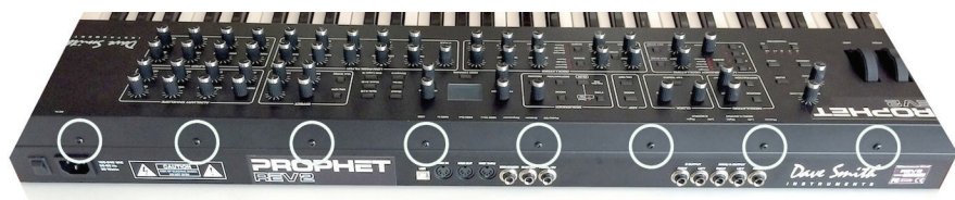
Remove the 8 screws on the back of the metal case
