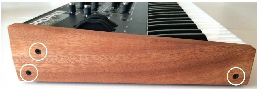
Remove the 3 screws from both the right and left wooden sides
