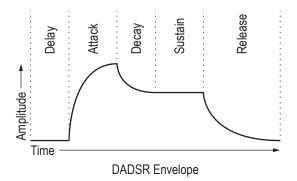
**Repeat:** Off, On—When on, the Delay, Attack, and Decay segments of the envelope repeat. Sustain still affects the level at which the Decay segment ends, but—instead of sustaining at a fixed level while a note is gated on—Delay, Attack, and Decay loop until the note is turned off. The Release segment begins when the note is gated off, just as it does when Repeat is off. See the illustration on the following page.
