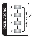
Use the four oscillator buttons to select an oscillator for editing. The arrows that connect the oscillator buttons is a graphic representation showing which oscillator affects another when the Sync, FM (frequency modulation), or AM (amplitude modulation) parameters are used. Oscillator 2 affects oscillator 1, oscillator 3 affects oscillator 2, and so on. For information about what the Sync, FM, and AM parameters do, see the relevant items later in this section.
