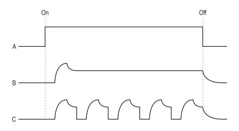
A: The gate generated by pressing, holding, and then releasing a key.
